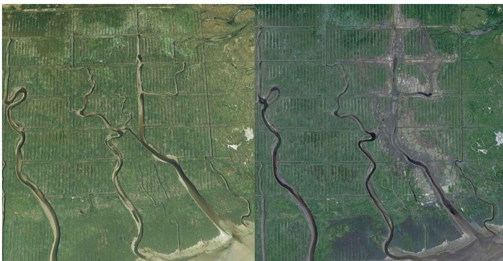
Figure 10. Restoration of natural drainage in the back-barrier salt marsh on island of Norderney, Lower Saxony. The top soil was removed to decrease the artificial drainage
