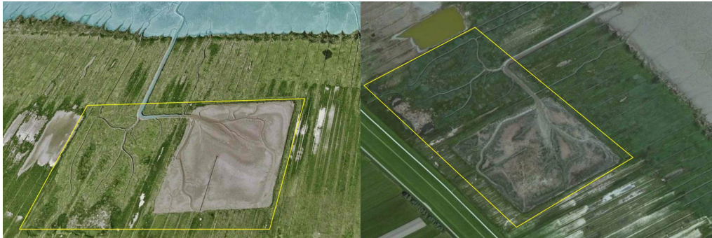
Figure 14. Clay extraction according to the traditional method in the salt marsh of the Jadebuse near Dangast, Lower Saxony. Left: Aerial view in 2000 on a 38-year old clay pit and a one-year old clay pit side by side. In both pits, a natural-like dendritic creek system developed (Photo: 2017 GeoBasis-DE/BKG on Google Earth); Right: same clay pits about 15 years later with establishing vegetation in the youngest clay pit (Photo: 2017 Earthstar Geographics SIO on Bing Maps by Microsoft).
